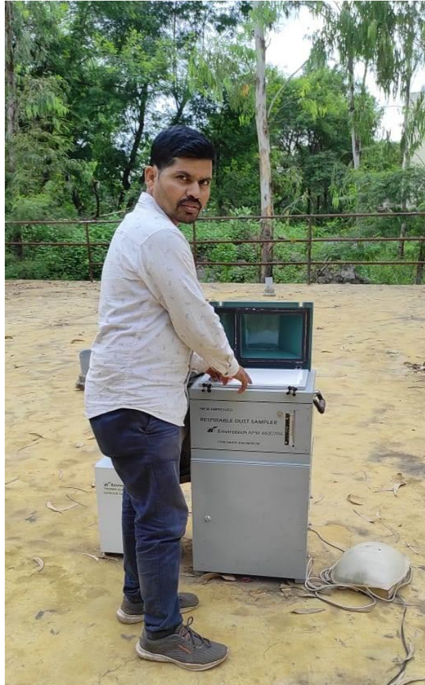
Shri.Amol Vyawhare and Shri. A.R.Swami Changing Filter Paper for RSPM at Monitoring Station C M.I.D.C.
