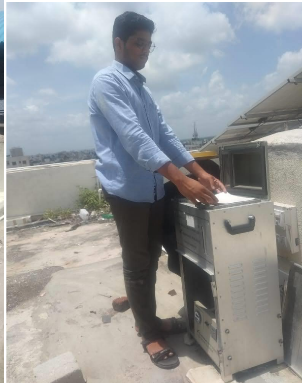
Mr.Prasad More and Niranjn Bansude changes filter paper on RDS machine at Monitoring Station A
