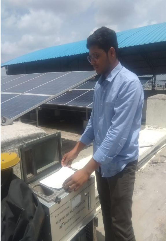
Mr.Prasad More and Niranjn Bansude changes filter paper on RDS machine at Monitoring Station A
