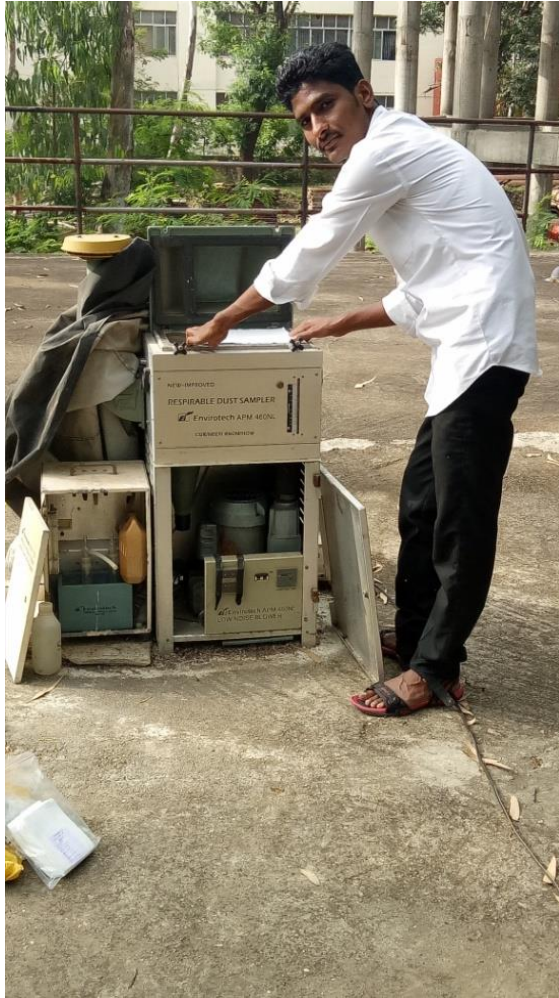
Shri.Amol Vyawhare and Shri. A.R.Swami Changing Filter Paper for RSPM at Monitoring Station C M.I.D.C.
