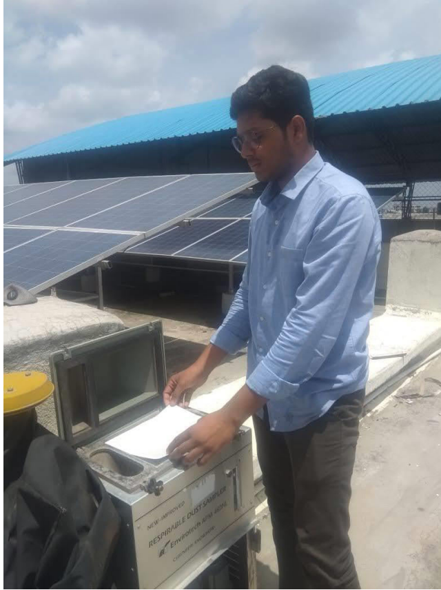
Mr.Prasad More and Niranjn Bansude changes filter paper on RDS machine at Monitoring Station A
