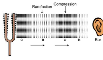
Fig.12.1: Compression and rarefraction of sound wave
