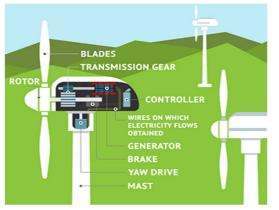
Windmills and wind turbines are different. They both use wind as a resource, but wind turbines are used to generate electricity. A wind turbine is a machine for converting the kinetic energy in wind into mechanical energy. Turbines and generators are equally used in the production of electric power; nevertheless, the turbine converts available energy forms into the rotation while the generator converts rotation into electricity. Two types of modern wind turbines generate electricity
