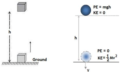
Consider an object of mass, 'm'. Let it be raised through a height, 'h' from the ground. The minimum force 'F' required to raise the object is equal to the weight of the object, 'mg'. The object gains energy equal to the work done on it. Let the work done on the object against gravity be 'W', given by,
