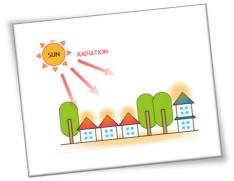
The transfer of heat from one place to another in a straight line with the speed of light without heating the intervening medium is called radiation. For transfer of heat by radiation, molecules are not needed i.e. medium is not required. The fact that earth receives large quantities of heat from the sun shows that the heats can pass-through space between the sun and the atmosphere that surrounds the earth. The transfer of heat by radiation has the same properties as light.
