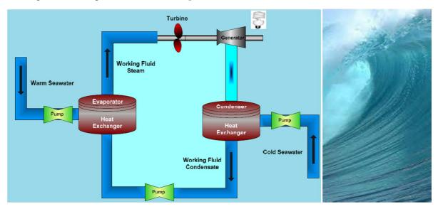
Fig.18.3: The OTEC closed cycle
