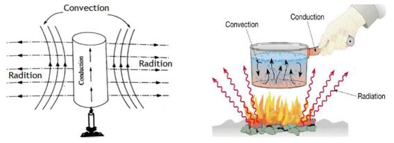
The figure shows heat transfer by conduction, convection, and radiation. The steel bar is heated by conduction. However, the bar loses heat by convection and radiation. The following **Table.11.1** describes the comparison between conduction, convection, and radiation.
