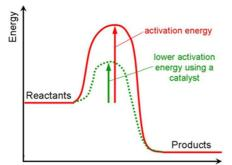
The role of catalyst in any chemical transformation cannot be neglected. A catalyst increases the rate of the chemical reaction by decreasing the amount of activation energy. Hence, we can save energy input and time to carry transformation. In summary, chemical energy makes its ubiquitous presence in the world's energy supply. It is so readily available and is found in nearly everything we use. At the same time meeting, the
