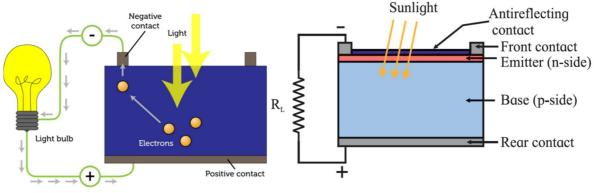
Fig.4.2: Structure of solar cell
