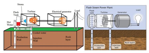
Fig.15.2: Flash steam geothermal power plant
