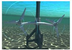
seawater instead of building a separate structure as in tidal barrages. These turbines are similar to wind turbines but are much larger because of the higher energy density of seawater compared to air. Storms do not affect tidal turbines just like wind turbines because they are installed below the surface. However, they have small diameters and higher speeds.
