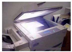
For a photocopier to work, a field of positive charges must be generated on the surface of both the drum and the copy paper. These tasks are accomplished by the corona wires. These wires are subjected to a high voltage, which they subsequently transfer to the drum and paper in the form of static electricity. Toner is very important in the photocopier. Toner is dry ink, it is a pigmented liquid. Toner is a fine, negatively charged, plastic-based powder.
