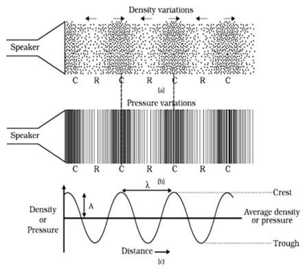
Fig. 12.2: Propagation of the sound wave
