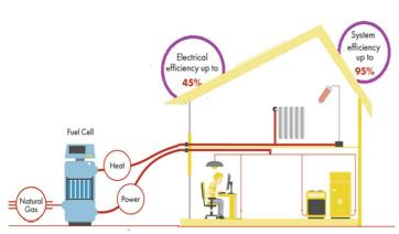
If, in addition to the generated electricity, the heat that is produced is also used, the process is referred to as combined heat and power (CHP). The fuel cell will produce electricity as long as fuel (hydrogen) is supplied, never losing its charge. Fuel cells are a promising technology for use as a source of heat and electricity for buildings and as an electrical power source for electric
