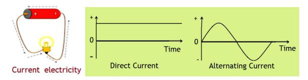
**Direct Current (DC):** It is an electrical current that flows consistently in one direction. Flashlight, Wall clock, Radio, etc. appliance running on batteries is direct current.Direct current is like the energy you get from a battery.
