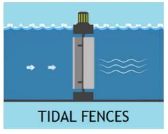
Tidal fences are also forms of tidal energy. They encompass vertical-axis turbines attached to the structure and water is forced through them which will then produce electricity. One of the main challenges is to transport tidal energy from underneath the sea to the grid and eventually to households. Other developing technologies seek to turn tidal energy into hydrokinetic energy which uses the same method of turbines beneath the sea.
