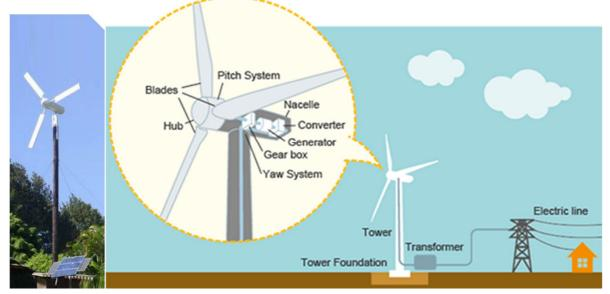
Fig.3.1: General Mechanism of wind energy generation
