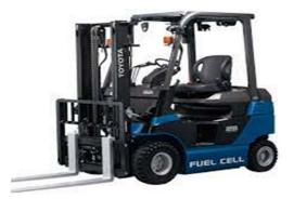
Fuel cell industrial trucks, like forklifts or towing trucks (airports), are especially suitable for indoor operation because they produce no local pollutant emissions and only low noise emissions. Fuel cell vehicles have advantages over battery-operated industrial trucks in terms of refueling. Instead of having to replace the battery, the trucks can be refueled within two to three minutes. They take up less space and are cheaper to maintain and repair.
