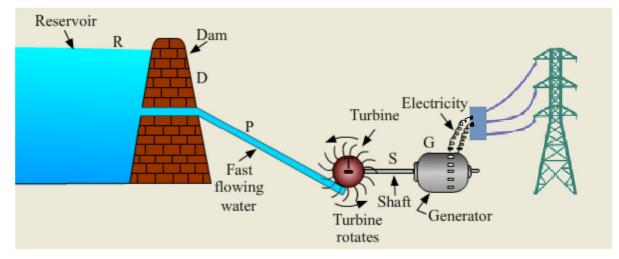
Fig. 16.2: Hydroelectric power plant
