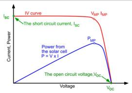
Fig.4.3: V-I characteristic of solar cell
