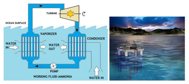
Fig. 18.1: Ocean thermal energy conversion system
