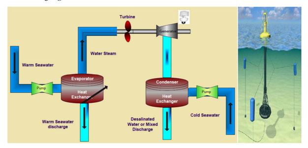
Fig.18.2: The OTEC open cycle
