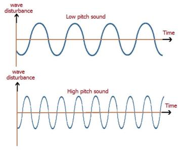
Fig.12.3: Low pitch and high pitch sound
