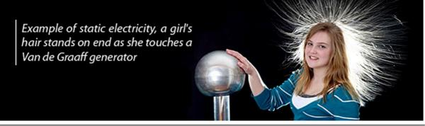
In 1929, Robert J Van-de-Graff designed in an electrostatic machine that is used to accelerate the charged particles e.g. protons, electron  $\alpha$ -particles, etc.
