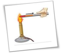
Heat passes through solids by conduction only. When one end of the metal rod is placed in a flame while others held in hand, the end being held becomes hotter and hotter, although it is not itself in direct contact with the flame. We say that heat has been conducted from hot end to cold end. Heat conduction can be visualized as the result of molecular collisions. As one end of the object is heated, then the molecules of the object vibrate faster and faster. As they collide their slow-moving
