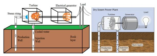
Fig.15.1: Dry steam geothermal power plant
