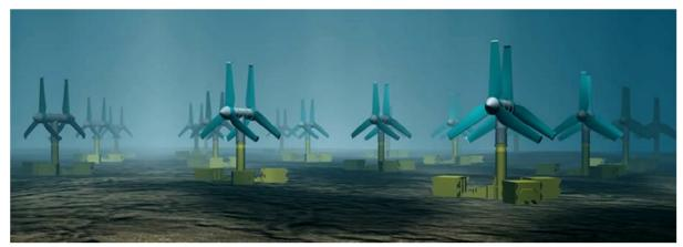
The supply of electricity from a tidal power plant will never match the demand on a system. But, due to the lunar cycle and gravity, tidal currents, although variable, are reliable and predictable and their power can make a valuable contribution to an electrical system that has a variety of sources. Tidal electricity can be used to displace electricity which would otherwise be generated by fossil fuel-fired power plants, thus reducing emissions of greenhouse and acid gasses.
