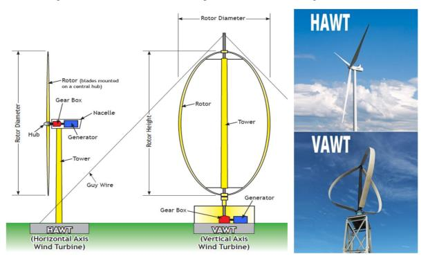
Fig.3.2: Schematics of HAWT and VAWT
