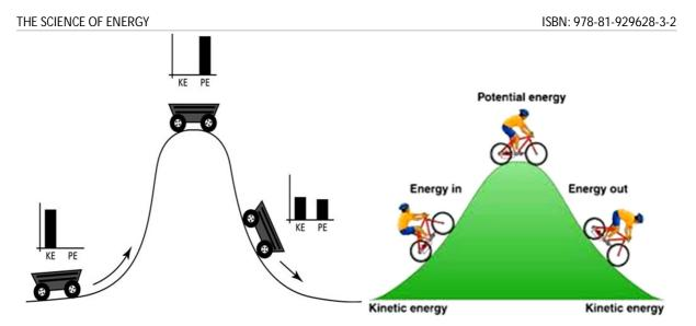
At the top of the hill, the car is pretty much stationary, so whereas all its kinetic energy is has been converted to potential energy. As the car begins its descent on the other side of the hill, the potential energy begins to be converted back to kinetic energy, and the car gathers speed until it reaches the bottom of the hill. Back at the bottom, all the potential energy the car had at the top of the hill has been converted back into kinetic energy.
