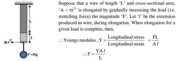
The magnitude of the force is not constant but changes from 0 to F during elongation of the wire. Let f be the force and x be the corresponding elongation then we can write,
