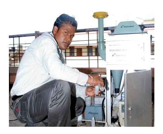
The Field Assistant Mr. Valmiki C.M. monitoring and collecting the sample So<sub>2</sub> & No<sub>x</sub> for laboratory analysis.
